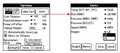
Select which vehicle you intend to scan by clicking on the appropriate box on the screen, as shown above. (Note that support for the L67 is only available with a combo LS1/L67 cable. Cables purchased before July 2003 may not have the new chip installed.) You can also click the Units button to change from default English units to Metric units.
